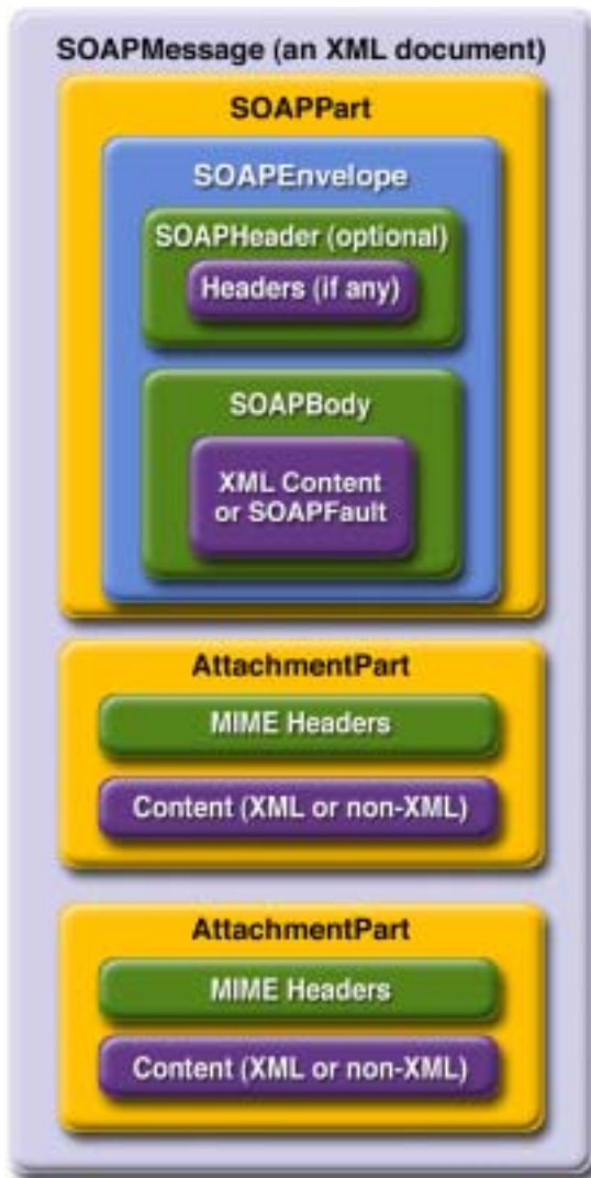
Figure 3–2 SOAPMessage Object with Two AttachmentPart Objects
